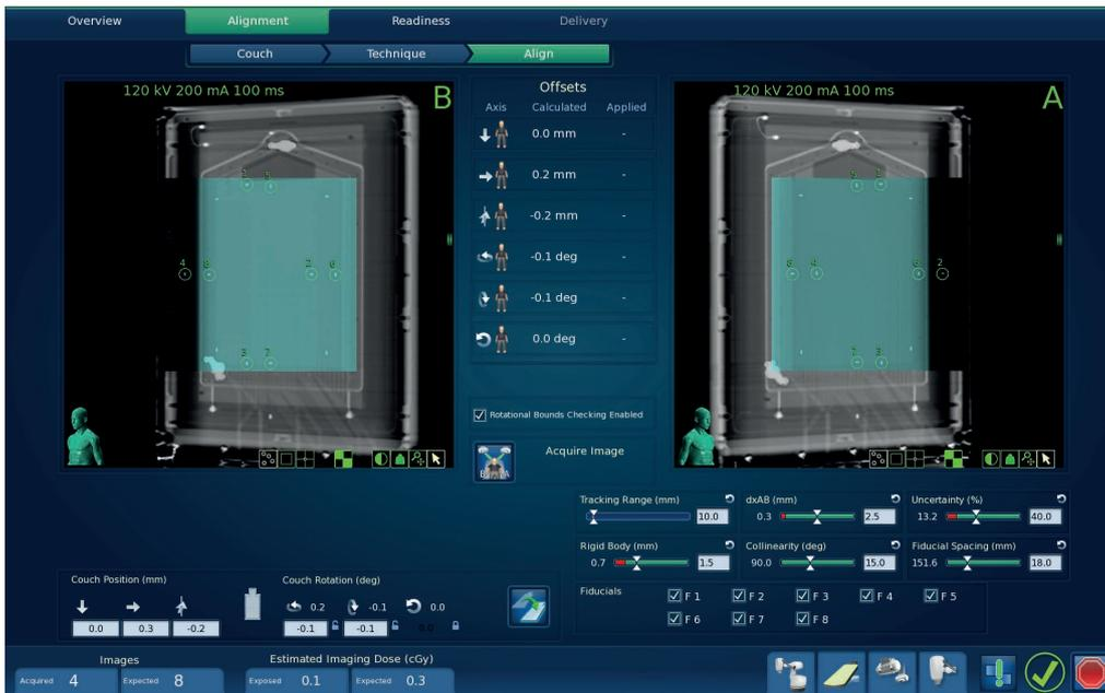
Figure 6: Automatic fiducial alignment
