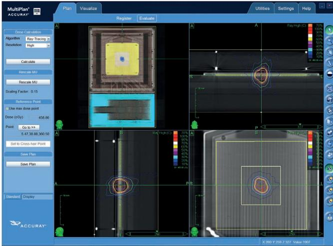
Figure 2: Patient QA plan alignment on the OCTAVIUS Detector
