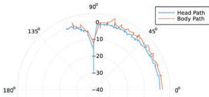
Figure 1: Angular response of the OCTAVIUS Detector 1600 SRS
