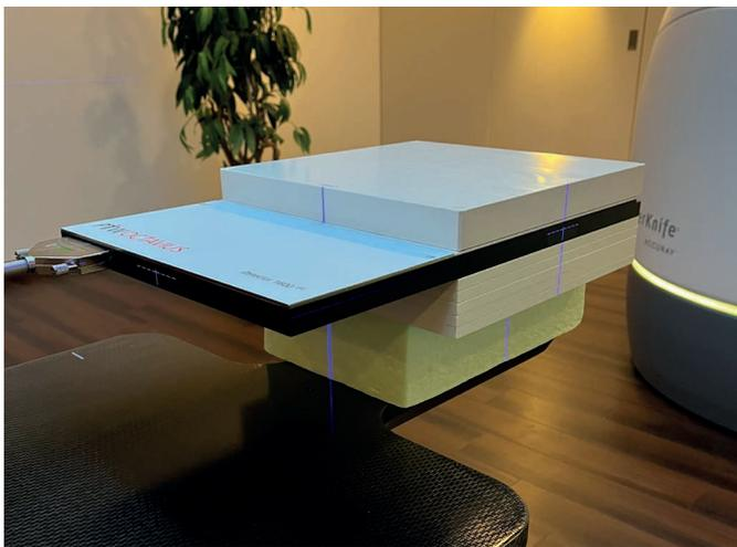
Figure 4: Measurement setup for patient-specific QA
