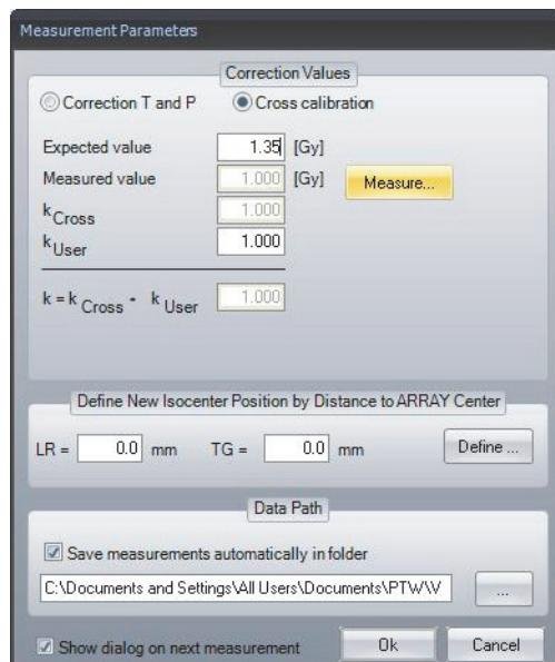
3. Perform the actual measurement using the above cross calibration factor.
