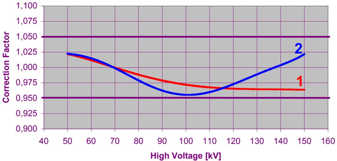
**Figure 1:** Typical energy response of the DIADOS detector for conventional diagnostic (1 - unattenuated beam, 2 - attenuated beam)
