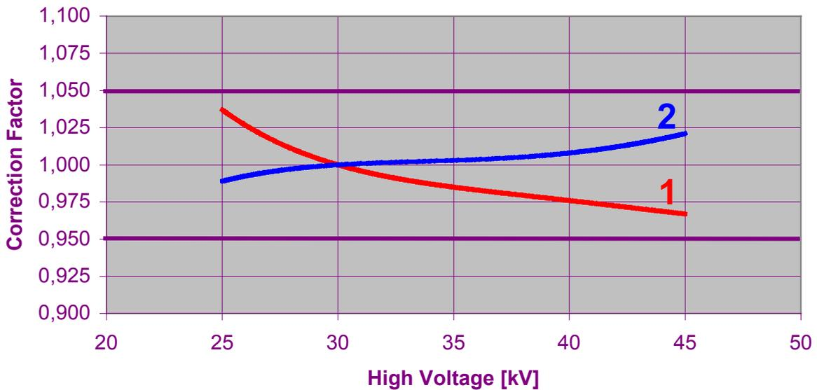
**Figure 2:** Typical energy response of the DIADOS detector for mammography (1 - unattenuated beam, 2 - attenuated beam)
