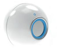
**QEYE** is a multi-layer detector for range and modulation verification in ocular tumor therapy. It is a device to measure depth dose curves to a depth of 60 mm WET. The resolution is 120  $\mu$ m resolution and the diameter of the sensitive area is 80 mm.
