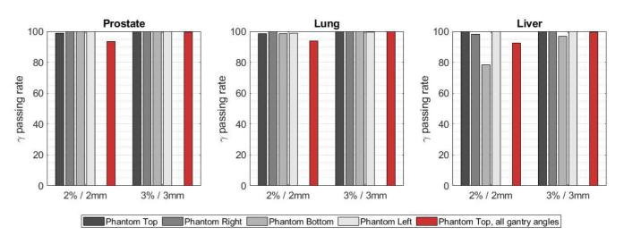
Figure 9: OCTAVIUS® 1600 MR array: Gamma passing rates for prostate, lung and liver treatment plans analyzed with 2 % / 2 mm as well as 3 % / 3 mm criteria. Grey bars show results of the split approach with different phantom positions and four QA plans, red bars show results of one measurement without different phantom positions.
