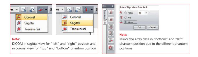
For the comparison between TPS calculation and measured dose in Verisoft, it is necessary to mirror the array data in "bottom" and "left" phantom position due to the different phantom and detector orientations. The TPS DICOM data must be displayed in sagittal view for "left" and "right" position and in coronal view for "top" and "bottom" phantom position, due to the different orientations of the array in each position.
