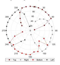
Figure 2: Angular response of OCTAVIUS® 1500 MR array in OCTAVIUS® II phantom. Phantom was aligned in four positions according to Figure 1.
