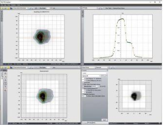
It can be observed in Figure 3, that the angular dependence of the OCTAVIUS® 1600 MR array in the phantom is very low. Due to this behavior, an additional approach was conducted to verify the patient plans without phantom rotation. For this purpose, the plan was irradiated to the OCTAVIUS<sup>®</sup> 1600 MR array in its original configuration in phantom "top" position
