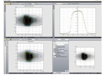
Figure 7: Comparison between measured plan with OCTAVIUS® 1600 MR array and calculated QA plan for measurement of all gantry angles with phantom "top" position. Comparison is shown for a TG profile analyzed with 3 % / 3 mm gamma criteria. First row left: prostate, first row right: lung, second row left: liver.
