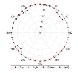
Figure 3: Angular response of OCTAVIUS® 1600 MR array in OCTAVIUS® II phantom. Phantom was aligned in four positions according to Figure 1.
