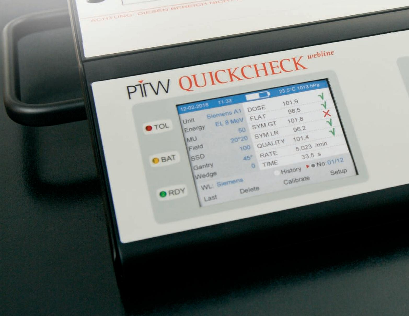
► Checks dose, dose rate, homogeneity, symmetry, beam quality,
