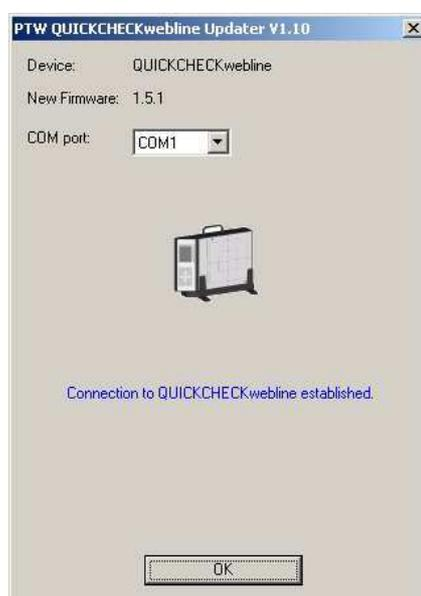
If the message is not displayed, try selecting a different COM port. Disconnect the power cable and turn off the QUICKCHECK<sup>webline</sup>. Make sure the RS232 connection between your PC and the device is established. Reconnect the power cable.
