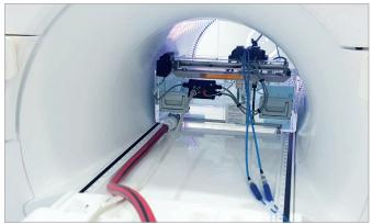
The system includes three 0.07 cm<sup>3</sup> Semiflex 3D ionization chambers. More **MR Conditional detector** types are available. Two models with vendor-specific water tanks for optimized scanning ranges are available:
