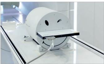
The OCTAVIUS 4D MR can be used with the MR Conditional array detectors **OCTAVIUS Detector 1600 MR** and **OCTAVIUS Detector 1500 MR**.
