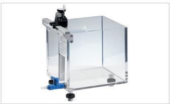
The **MP1 Manual MR** is an MR Conditional one-dimensional water phantom to measure dose in different depths. A radiation detector can be positioned in the water-filled phantom using a manually driven 1D moving mechanism. The measuring signal of the radiation detector is read out with an electrometer, e.g., the UNIDOS Tango. The tank has a vertical moving range of 254 mm and external horizontal phantom dimensions of 320 mm x 370 mm. A selection of **MR Conditional detectors** is available.
