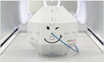
The System QA insert features MR visibility in T1 and T2 at 1.5 T and allows the positioning of an MR compatible detector in the center of RUBY. End-to-end QA can be performed using the adapt-to-position or the adapt-to shape workflow.
