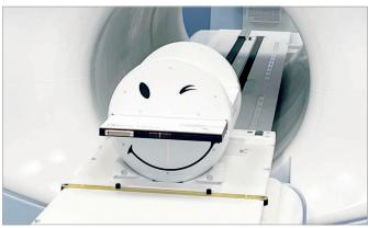
The **OCTAVIUS Detector 1600 MR** is the MR Conditional version of the OCTAVIUS Detector 1600 SRS. It is a liquid-filled 2D array detector. The very small detector size of only 2.3 mm x 2.3 mm x 0.5 mm makes this array detector ideally suited for small field dosimetry.
