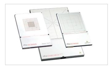
Apart from BEAMSCAN MR, machine QA in MRgRT may also be performed with our range of MR Conditional array detectors. With just one shot, all relevant beam data for radiation fields are delivered. Profiles are measured in real-time, making these array detectors an ideal tool for real-time beam tuning.
