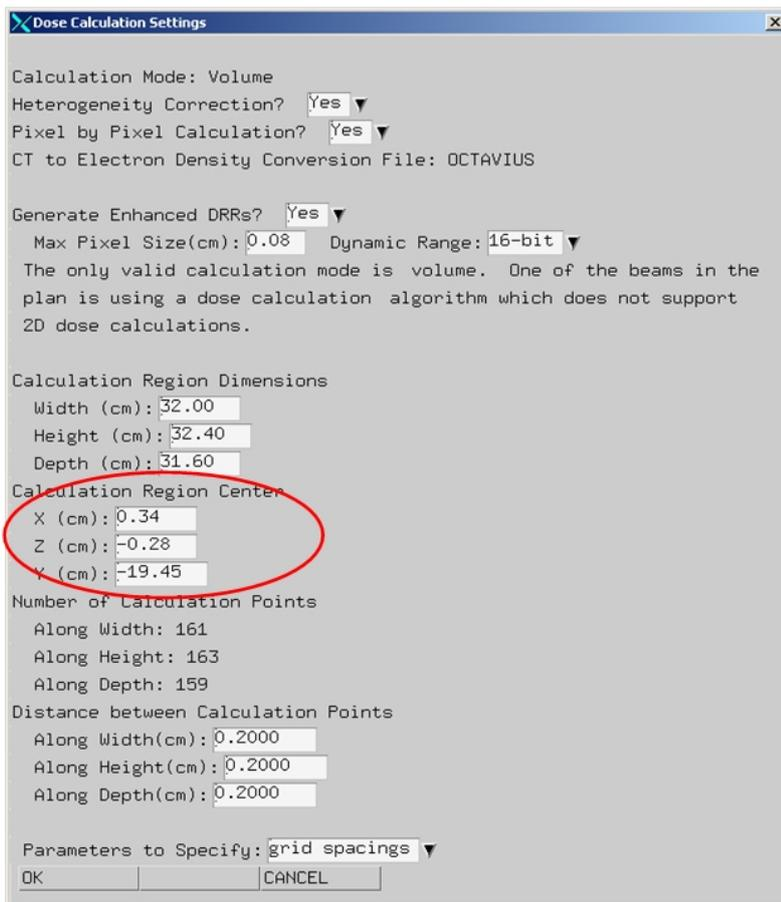
Figure 8 - Setting the "Calculation Region Center" in the "Dose | Calculation | Settings" dialog box
