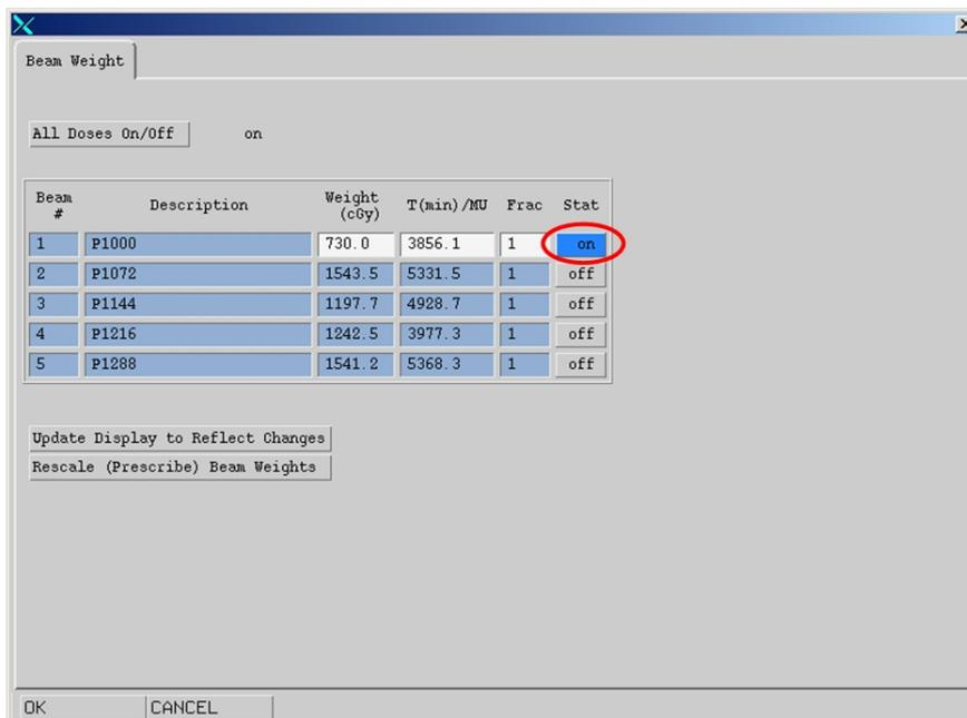
Figure 9 - Setting ON / OFF the treatment fields in the "Dose Weight" dialog box
