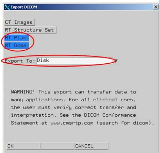
Figure 13: Selection of DICOM / DICOM RT objects to be exported and selection of destination ("Export To:" can be "Disk" or any DICOM SCP destination configured and then available in the drop-down list. In case of "Disk", the files are saved inside an XiO folder already shared on the network with a path like: \\<IP address of XiO work-station>\network\dicom\focus\_out
