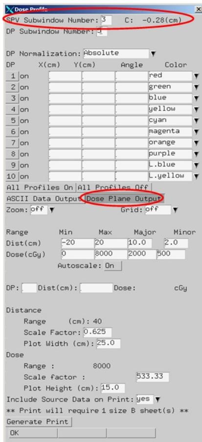
Figure 12 - Exporting a 2D dose matrix in ASCII text file format in the "Dose Profile" dialog box
