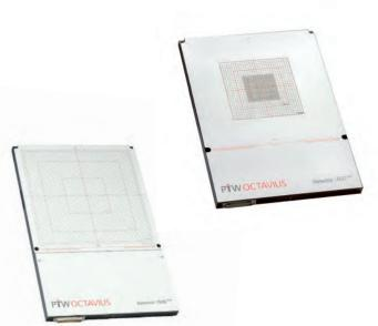
(1500 XDR) and 2.5 mm x 2.5 mm x 2 mm (1600 XDR) in size. The square chamber design of the OCTAVIUS Detector 1500 XDR offers 50 % field coverage and the design of the OCTAVIUS Detector 1600 XDR offers unique 100 % field coverage in the central region. Read out cycles of 100 ms provide the basis for real-time analysis of beam profiles.
