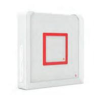
**NEXTQ** is an all-in-one, accurate device to speed up QA procedures by measuring beam characteristics (intensity and lateral profiles) in a single beam shot. It consists of x and y strip ionization chambers with a physical resolution of 1 mm, and an integrating chamber. The sensitive area is 127 mm x 127 mm.
