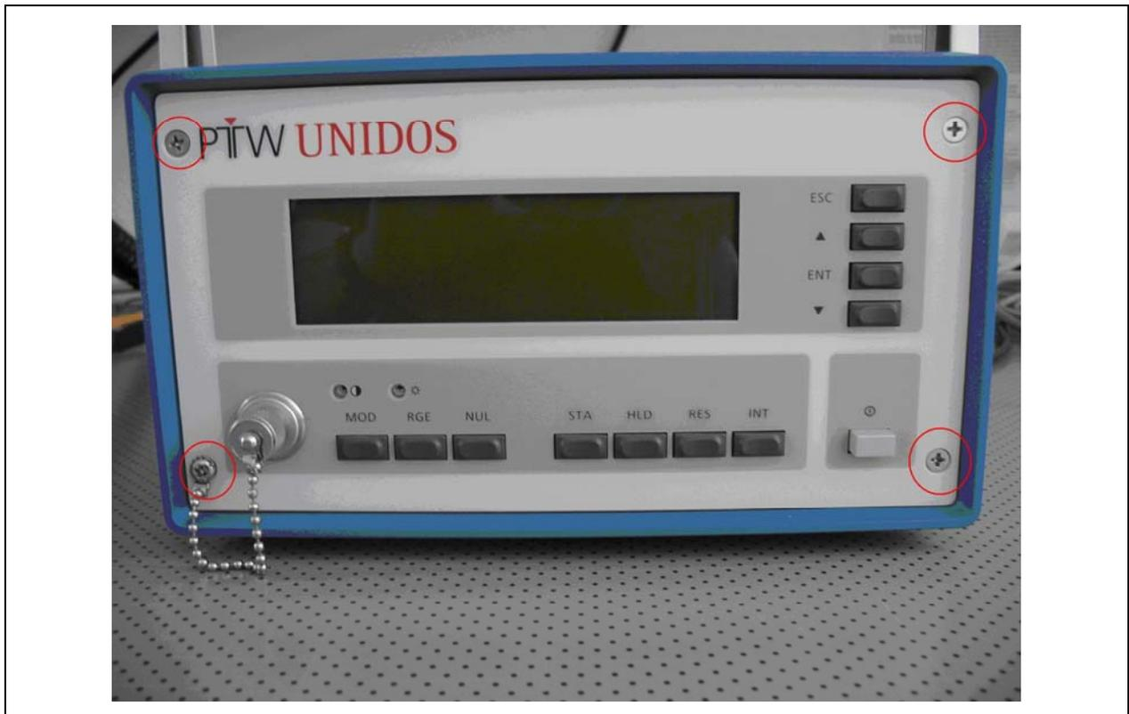
Figure 2: Position of the 4 screws on front panel
