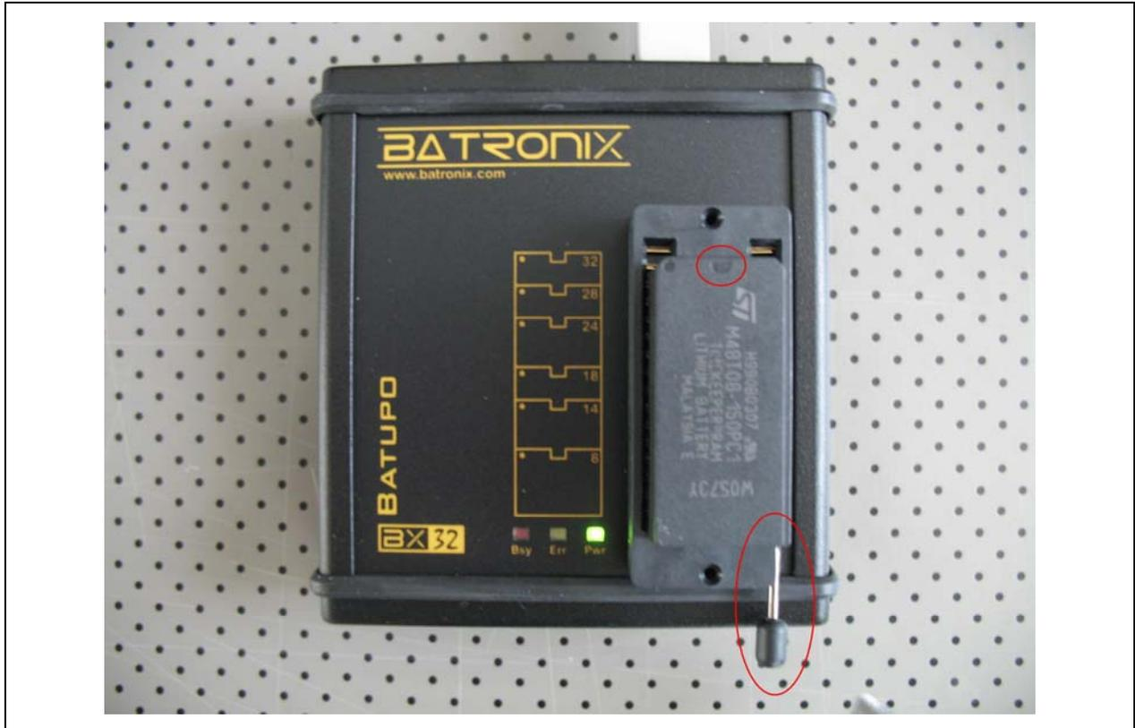
Figure 12: NVRAM inserted into the programmer; the mark of the chip and the lever are encircled
