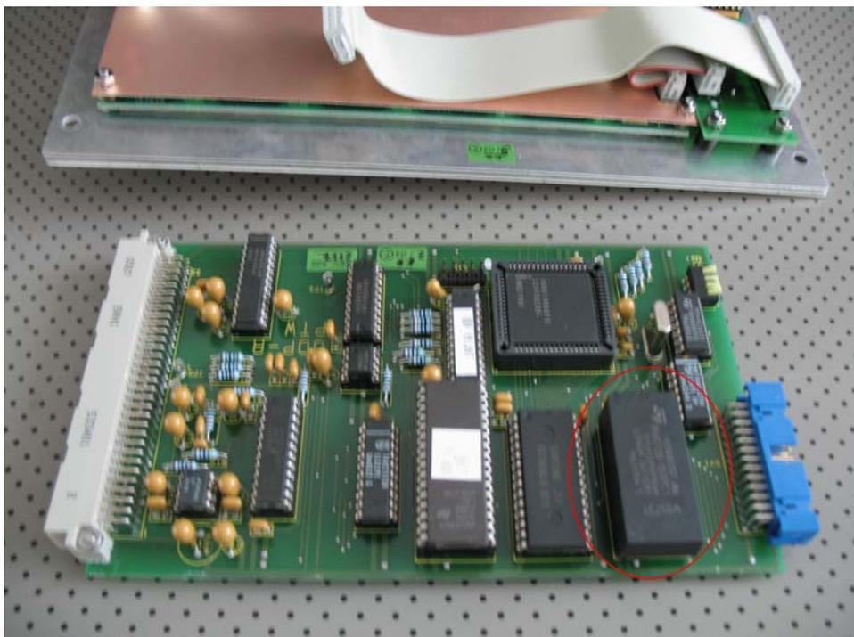
Figure 7: Printed circuit board with NVRAM
