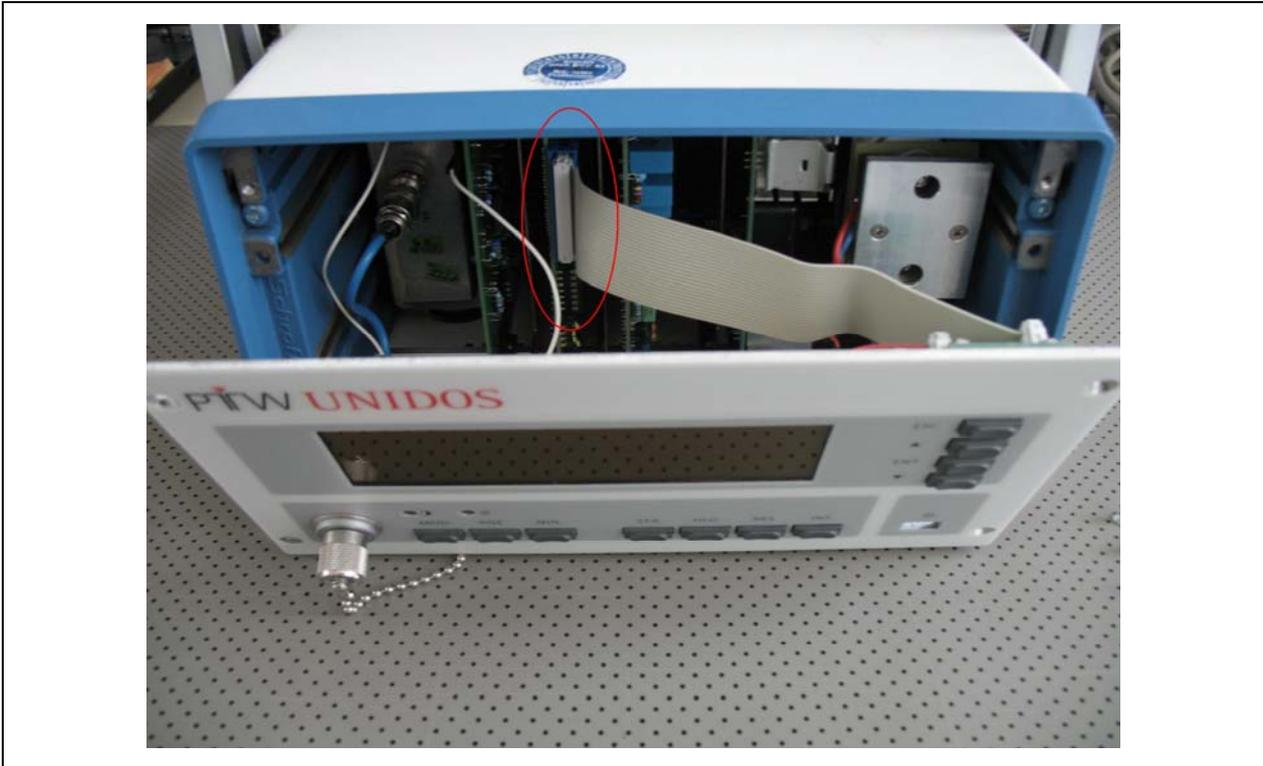
Figure 3: Flat ribbon cable attached
