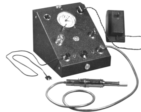
First PTW electrometer in 1922
