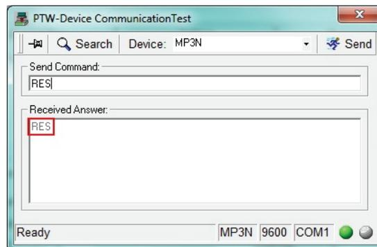
10. Turn the Control Unit off, wait 10 seconds, and turn it on again. The Control Unit is now reset to factory defaults.
