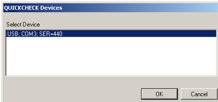
Check the serial number(s) of the device(s) in the **QUICKCHECK Devices** dialog (SER=...) to make sure your QUICKCHECK *webline* appears in the list. Select the device for which you want to set up the new connection. Click **OK**. WorklistGenerator software will automatically set up the connection.
